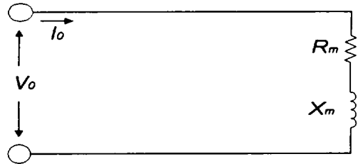
Fig. 6 Simplified no-load equivalent circuit.
