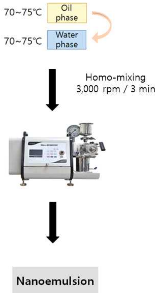
Figure 5. Manufacturing process of nanoemulsions by high-pressure homogenization method.
