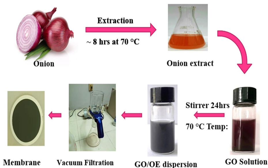
Figure 6. Modification of GO with onion extractive and Quercetin powder, and fabrication of GO/OE, and GO/Q composite membranes respectively.
