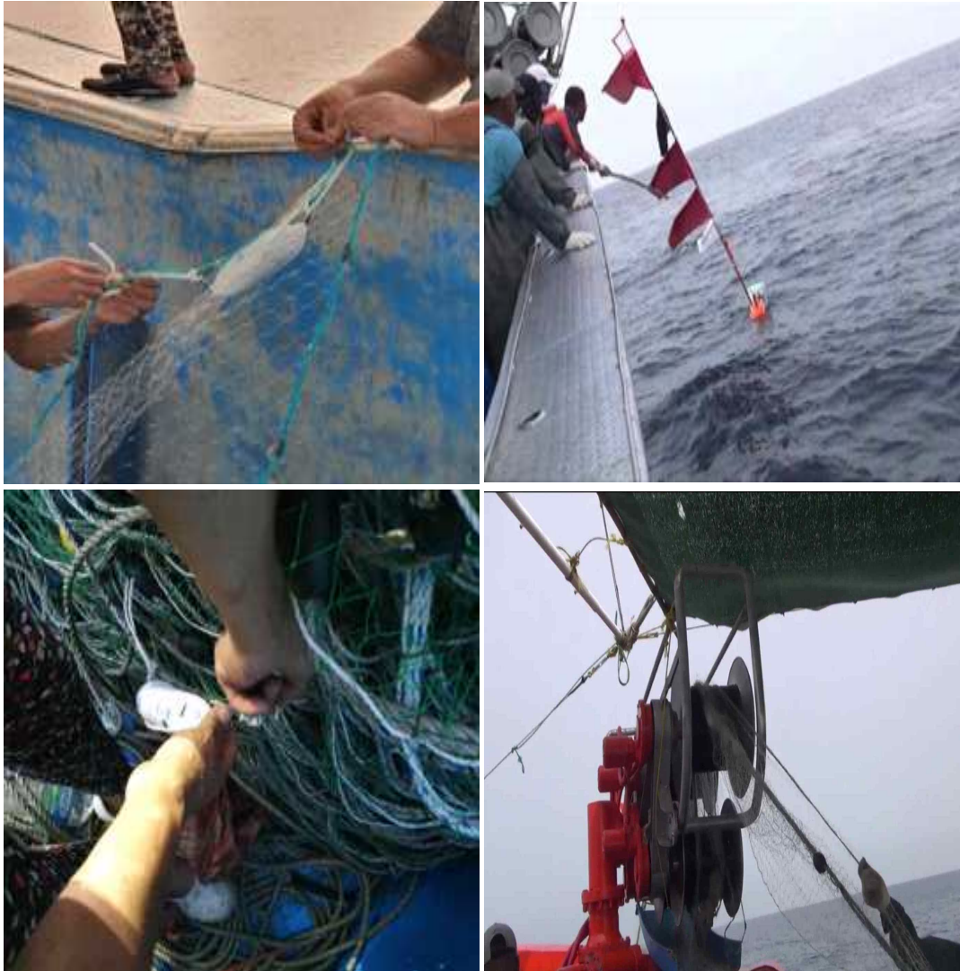
Fig. 3-5. Field test scene of the automatic fishing gear identification device underwater transmitter attached to the drift net fishing gear.
