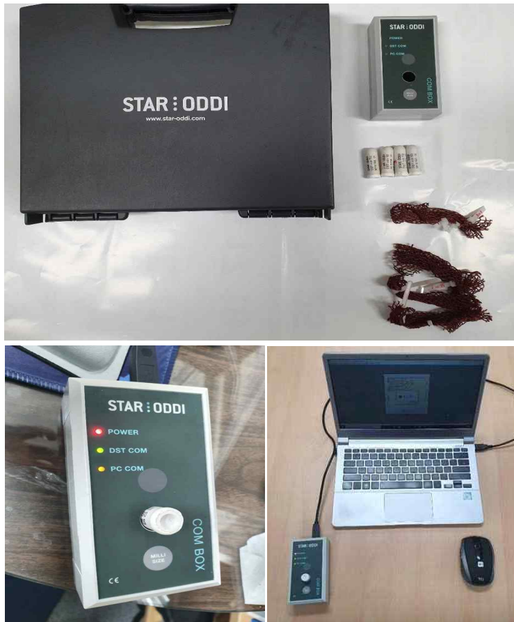
Fig. 2-4. Depth measuring instrument used for depth measurement analysis (Dst milli-TD, Staroddi)
