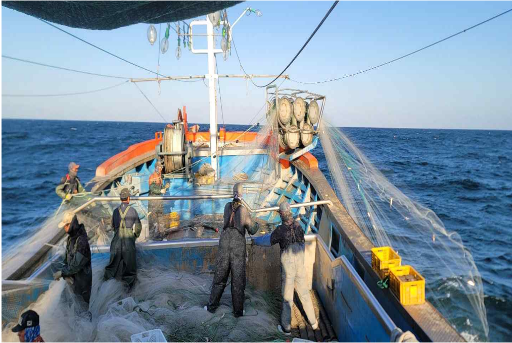
Fig. 1-9. A scene of operation using a net hauler of 5 step.
