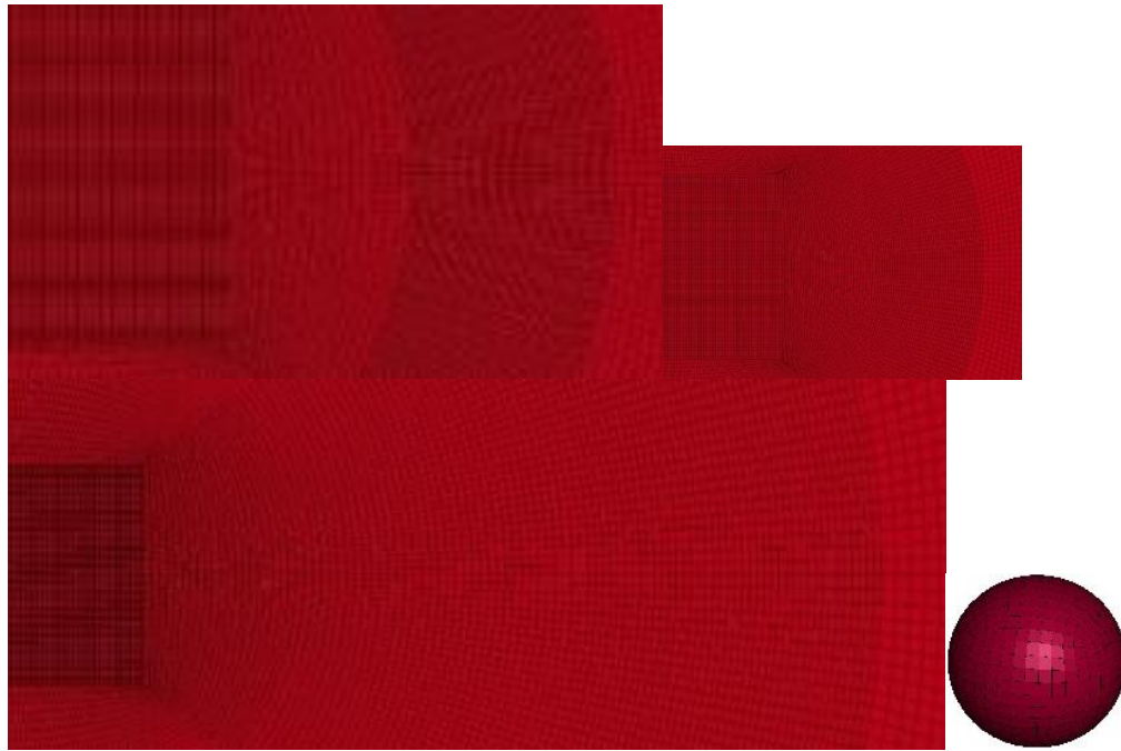
Figure 21. Finite element model for SPIF process
