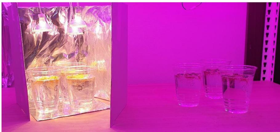
**Figure 2. Photo of temperature reaction experiment. L: LED bar+halogen lamp. R: LED bar (Control).**
