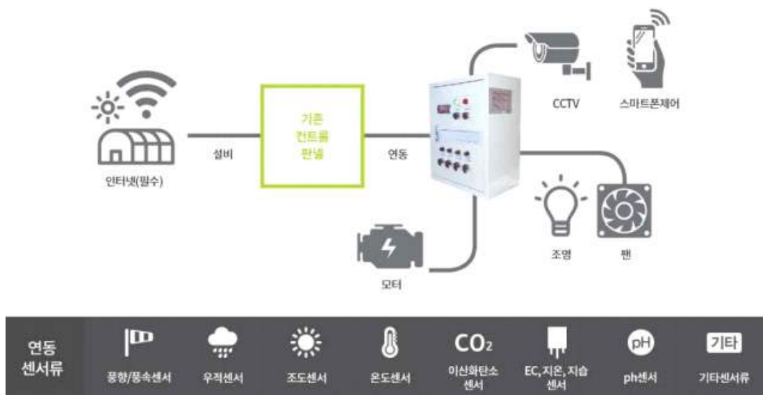
Fig 7. Farm Labs Smart Farm Configuration Diagram
