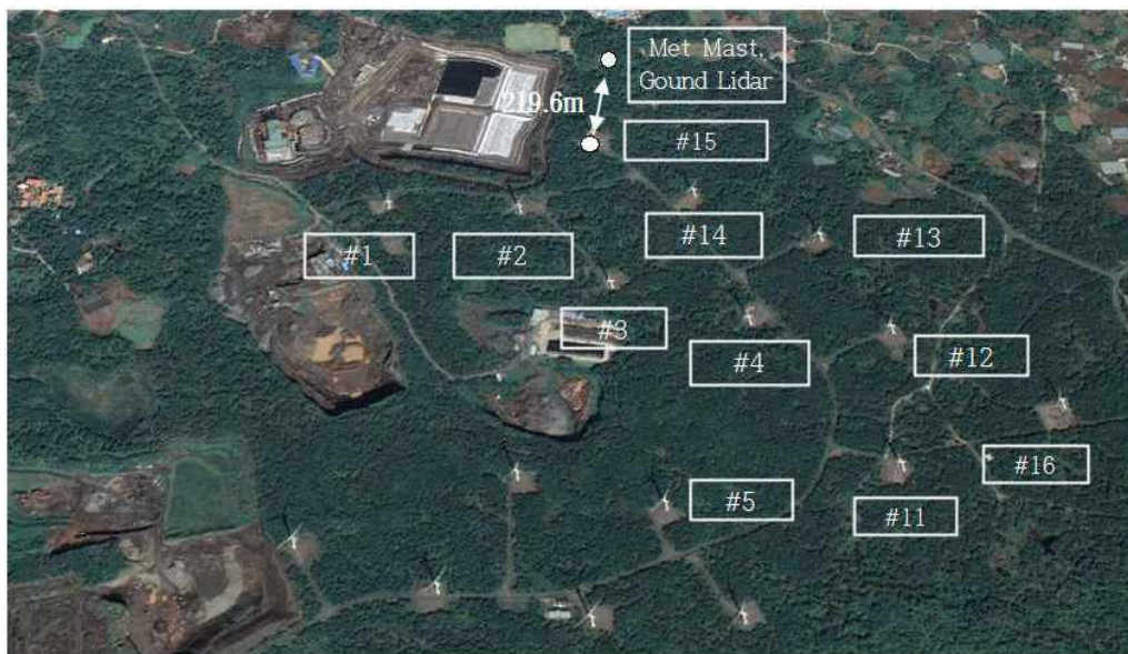
Fig. II-2 Layout of Dongbok wind farm
