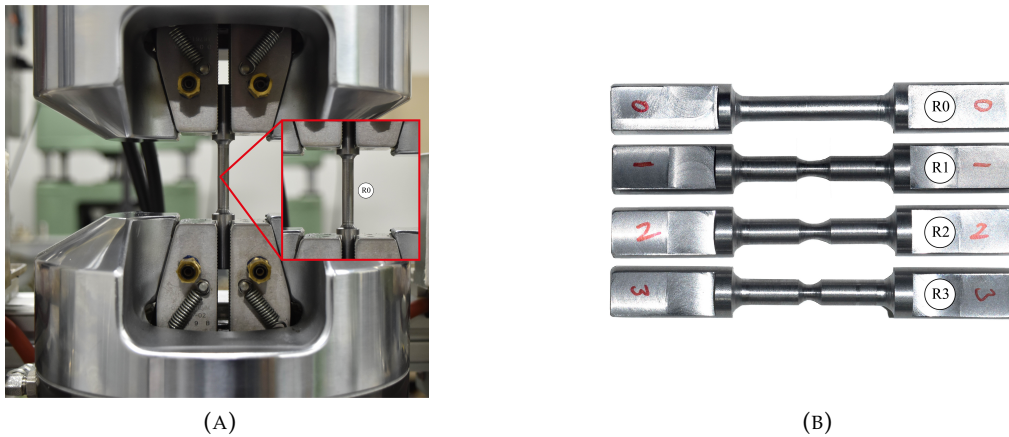
FIGURE 2.4: Experimental set-up to perform tension test at room temperature. (a) Test machine; (b) Un-notched and pre-notched specimens.
