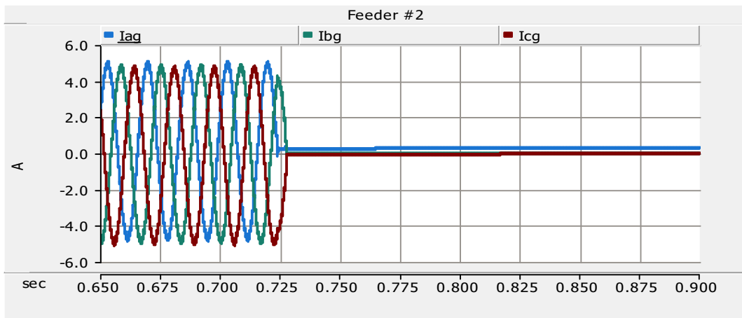
Fig. 24 Case 1-2 simulation result: Current of the normal feeder in the PCS source
