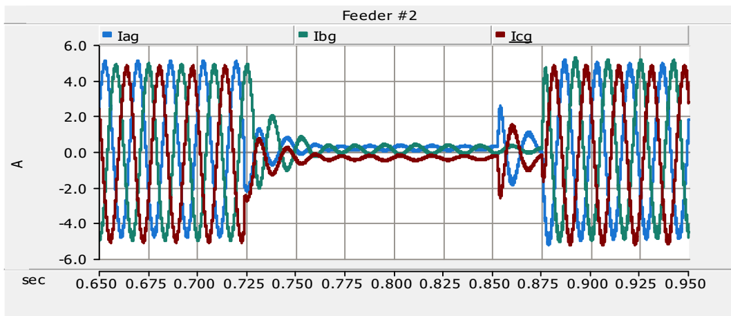
Fig. 50 Case 2-3 simulation result: Current of the normal feeder
