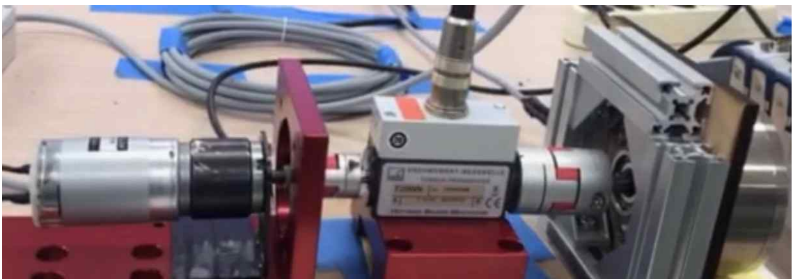
Figure 30 Particle brake torque measurement
