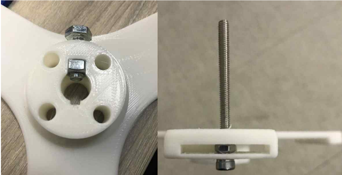
Figure 14 Blade fixture detail
