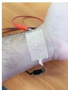
Figure 4-10 Wrist pulse rate measurement using custom made board
