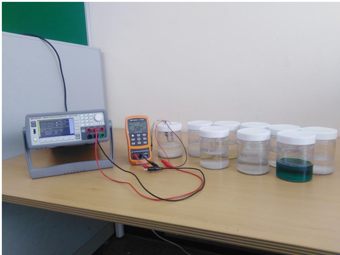
Figure 10, Setup used for measuring electrical response w.r.t RH%.
