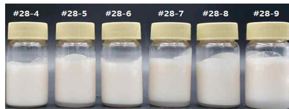
Figure 13. Phase separation of the PLO gel in which the liquid crystal formed at 5 °C, day 1.
