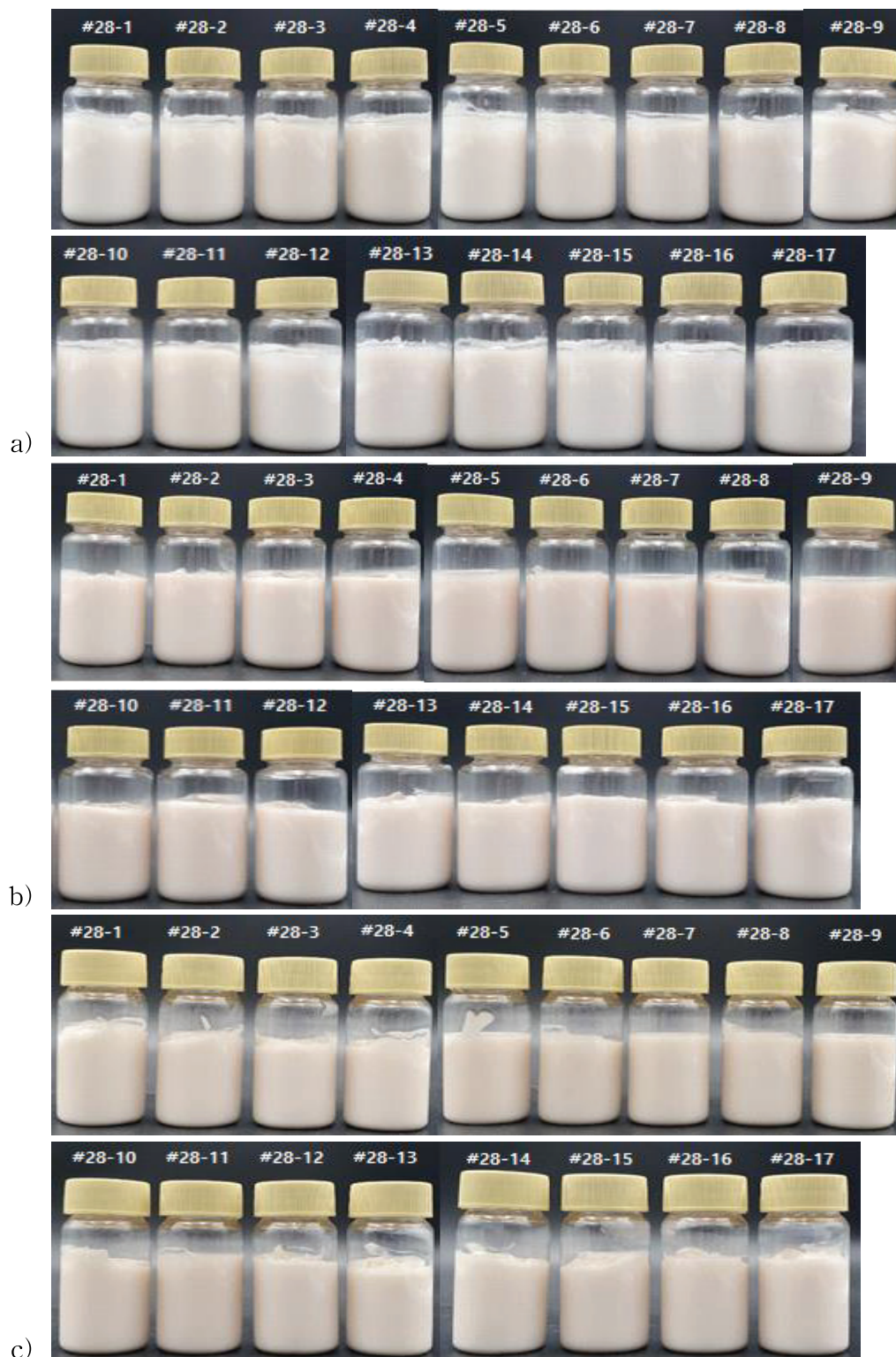
Figure 14. State of the PLO gel with different composition according to temperature and time. a) 25 °C, day 1, b) 25 °C, week 2, c) 40 °C, week 2
