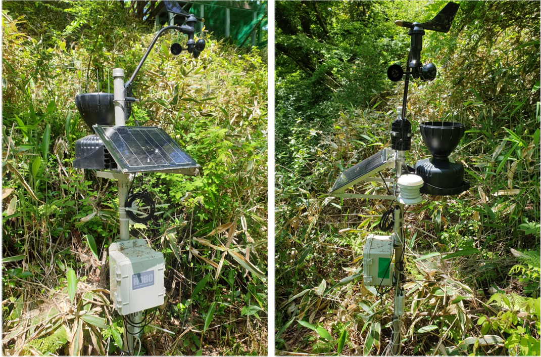
Fig. 2. HOBO: Research-grade data logging weather station on-board LCD display in a rugged.
