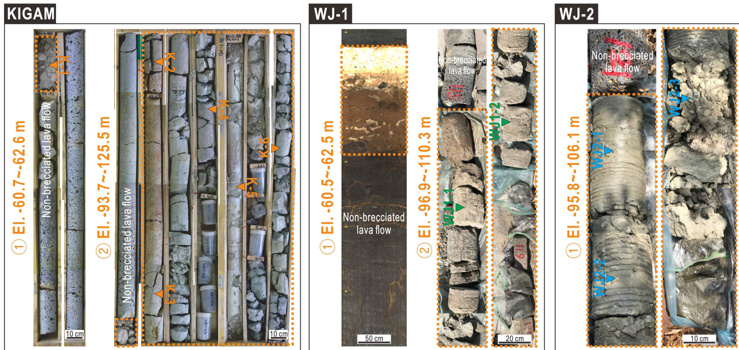
Fig. 4-8. Photos showing non-volcanic sedimentary rock intervals of borehole core and OTV logs. Triangles indicate sampling points for grain-size analysis.
