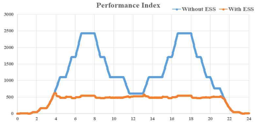
Fig. 5.22 Comparison of the performance index in discharging mode
