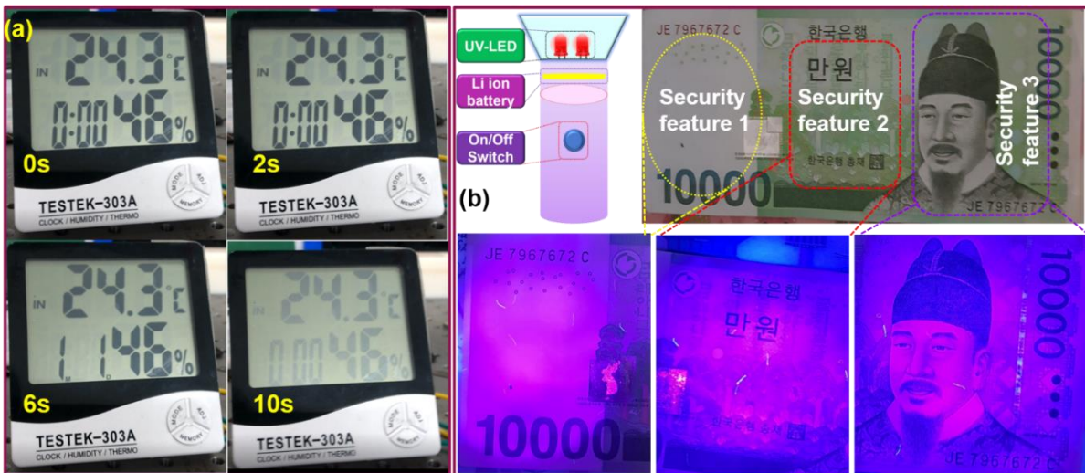
Figure 6.12. (a) The lit-up of the temperature sensor for 10s with 100 \mu\text{F} capacitor. (b) The designed self-powered UV counterfeit system is showing the three different areas for the security feature under UV light.
