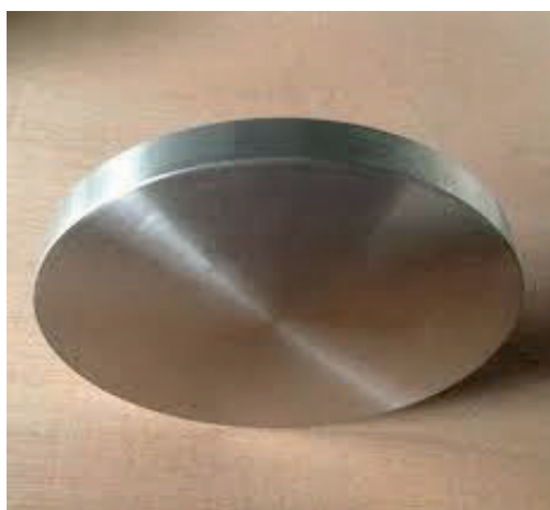
Figure 2. 5 Image of 2" diameter and 1/4 th " thick Zr target
