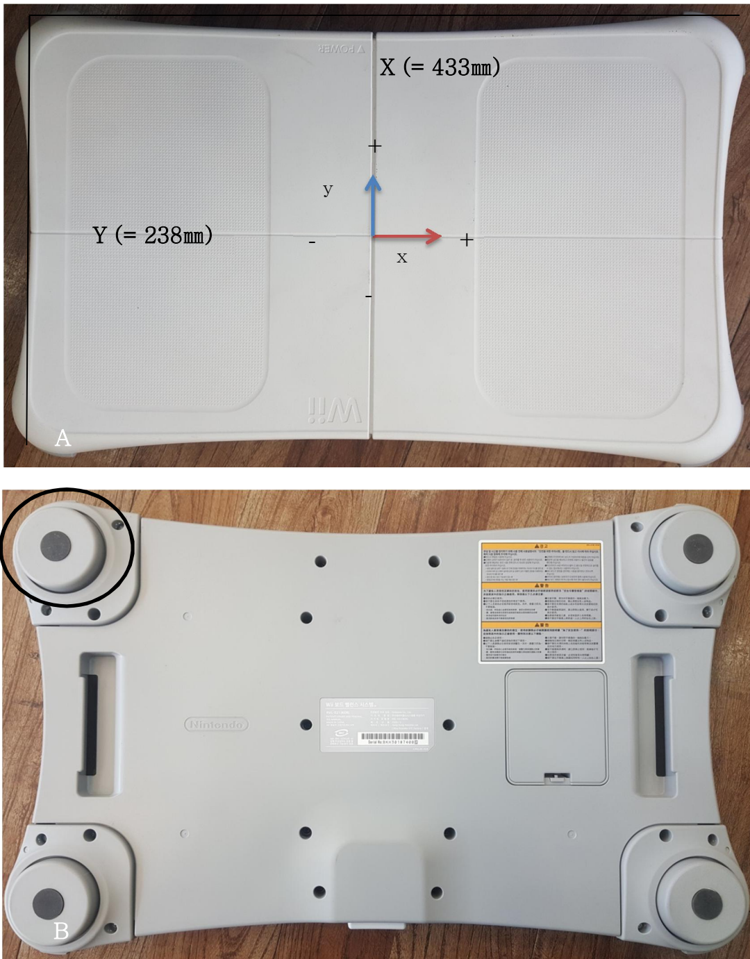
Figure 1. The WBB coordinate system and force transducers. (A) The x and y coordinates of the pressure center on the WBB are recorded for each frame. B) Foot-pegs housing force sensors (circle) are found under each of the four corners of the board as a uni-axial force transducer.
