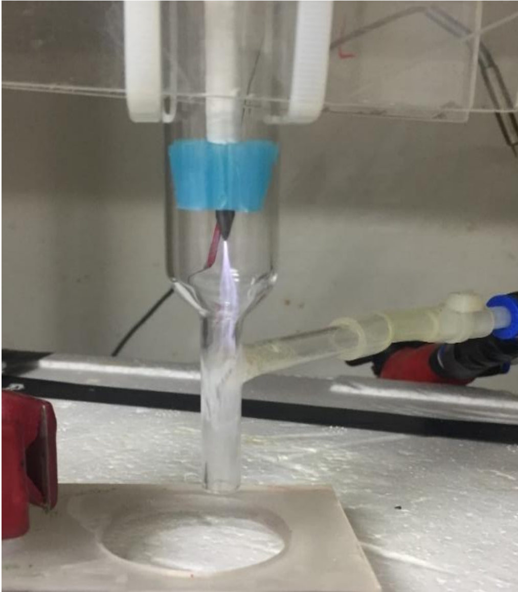
Figure 1.1.1. Typical corona discharge photographic image.
