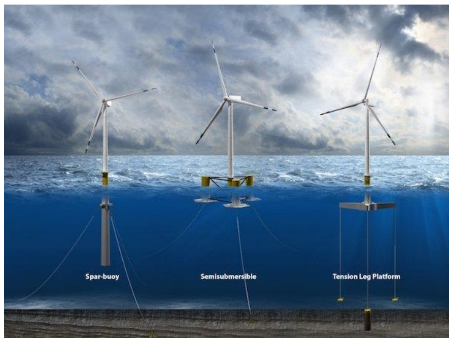
Fig 1-4. The floating foundation of offshore wind turbine
