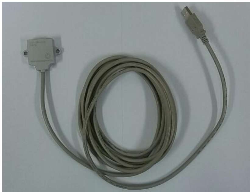
Fig. 6 Photo of the inclinometer
