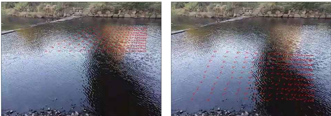
Fig. IV-35. Result of velocity vector in Jungmun-stream using Surface Image Velocimetry(SIV)
