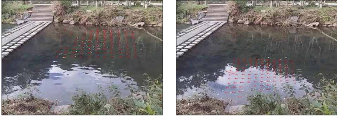
Fig. IV-41. Result of velocity vector in Yeonoei-stream using Surface Image Velocimetry(SIV)
