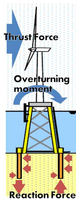
Fig. 1.3 Applied loads and reaction force on support structure for OWT (Moon and Park, 2018)
