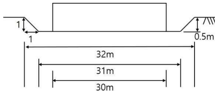
Fig. 3.12 Basic facility sectional view
