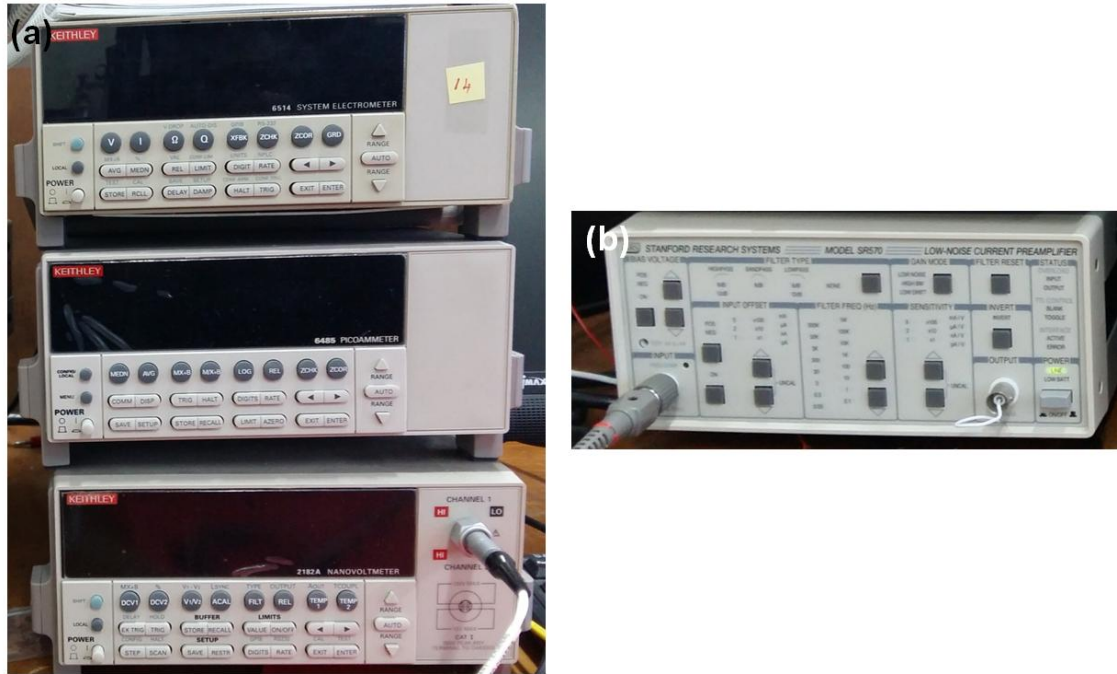
Figure 2.4 (a) Keithley measuring instruments such as 6514 electrometer, 6485 picoammeter and 2184 A nanovoltmeter (b) low noise current preamplifier.
