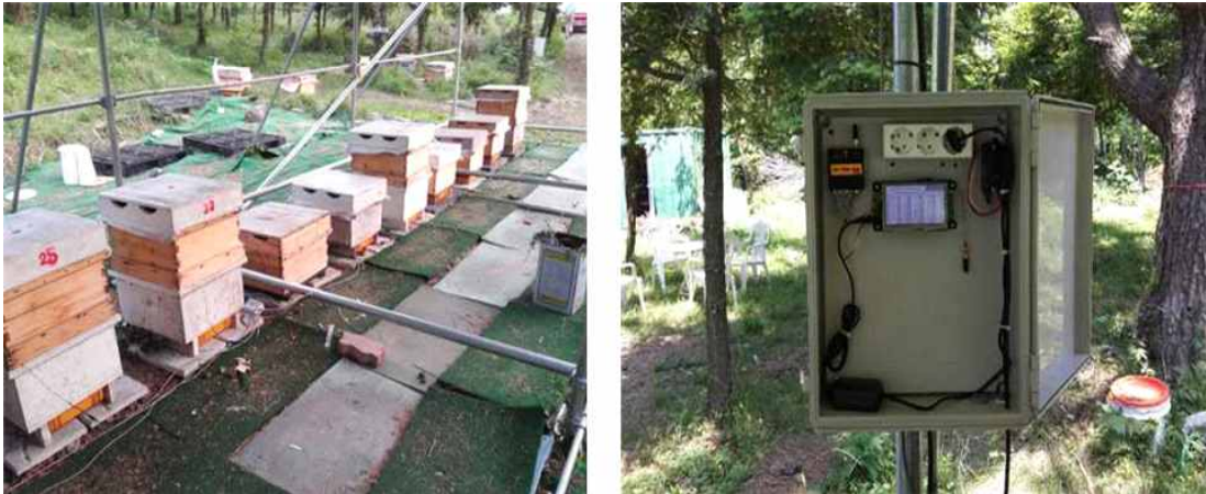
Fig. 21. Beehive with Sensor Board(Left), Installed Communication Board(Right)
