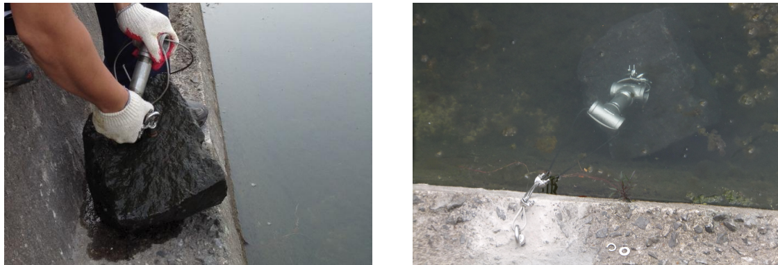
Fig. III-19. The position of DIVER-water gauge
