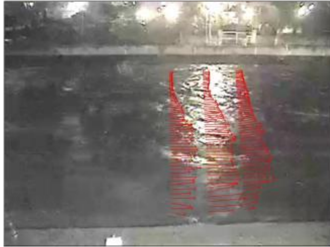
Fig. IV-12. Result of flow velocity vector for SIV (night-time).
