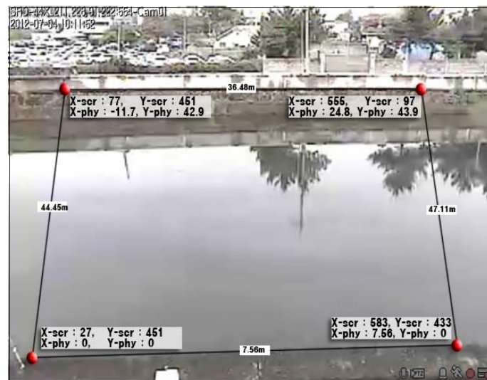
Fig. III-17. Reference point for Image coordinate transformation.
