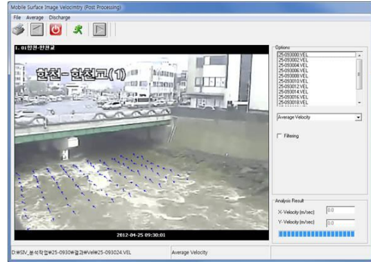
Fig. II-2. Analysis of SIV process; a) process of setting the default; b)reference point setting; c) Program Set analysis section(Create a grid network); d) Velocity vector
