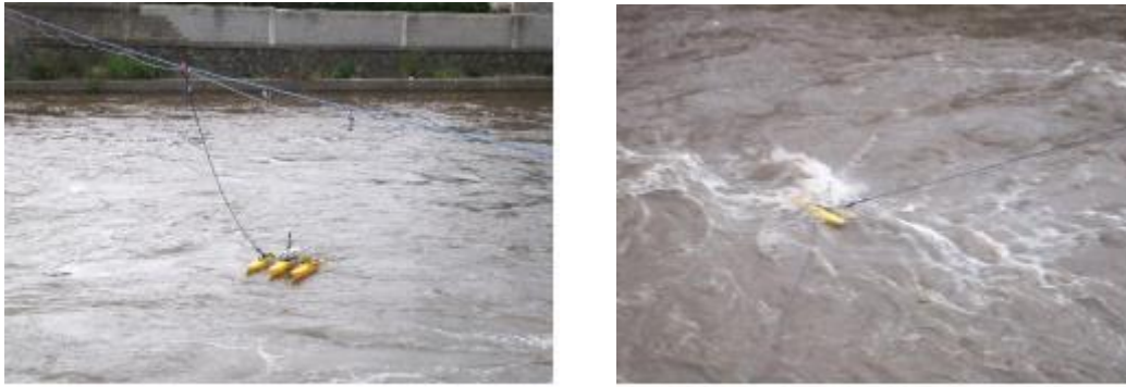
Fig. III-20. Discharge observation method using the ADCP
