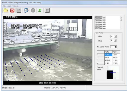
Fig. II-2. Analysis of SIV process; a) process of setting the default; b)reference point setting; c) Program Set analysis section(Create a grid network); d) Velocity vector
