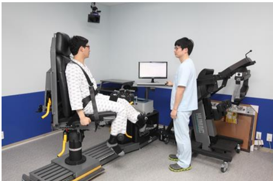
Figure 1. The figure shows the muscle isometric strength test with an isokinetic dynamometer
