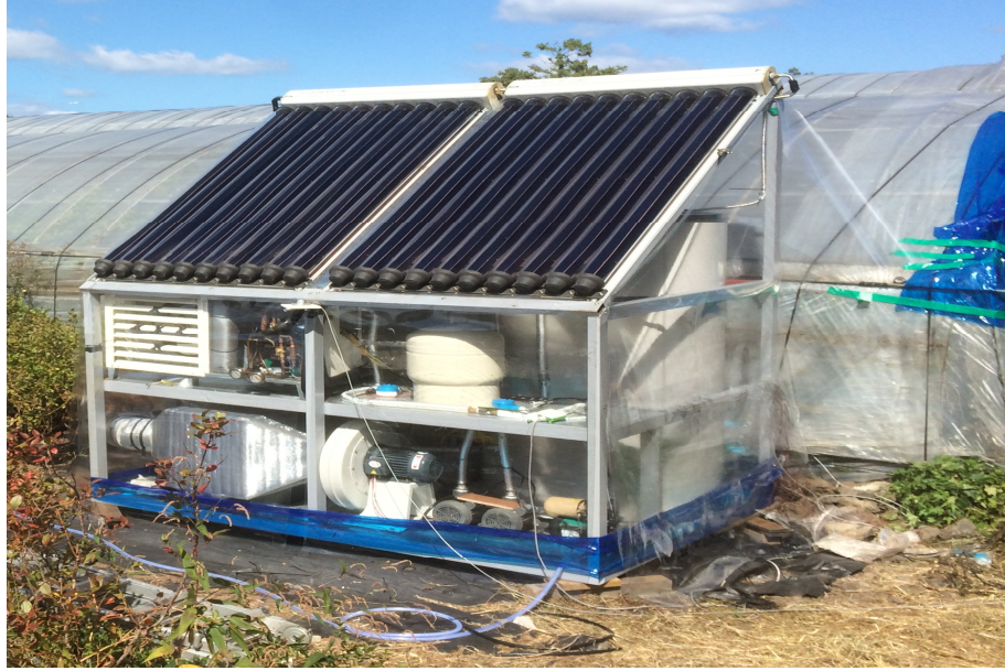
Fig. 9 Picture of thermal storage type hybrid heat pump system
