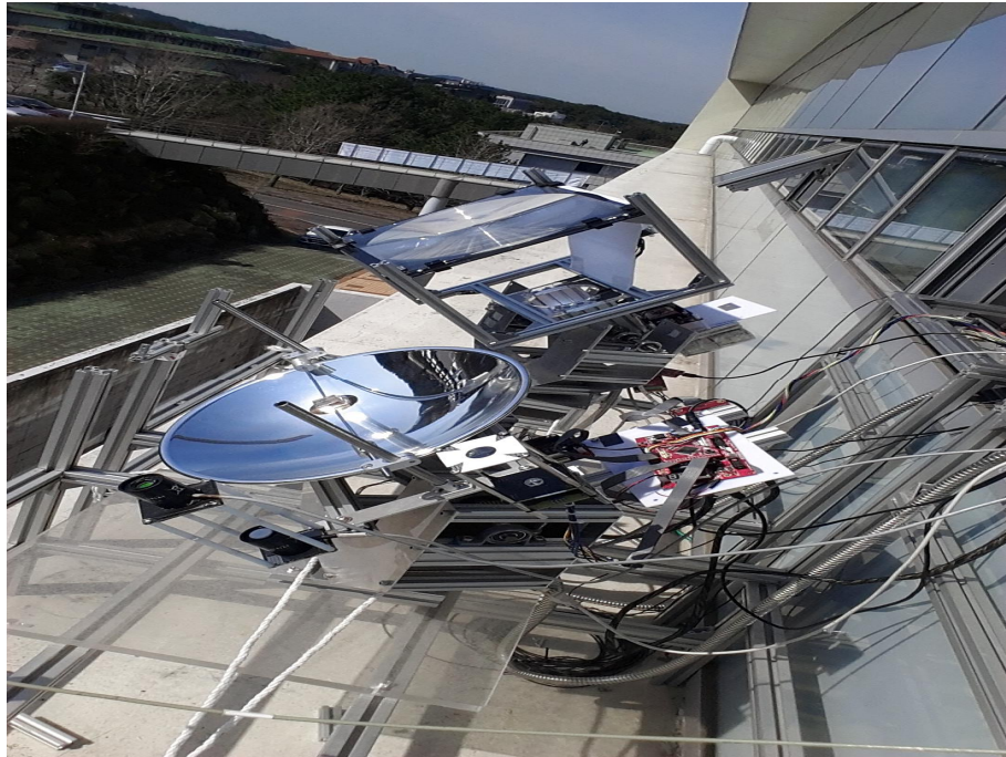
Fig. 62. Solar tracking system using Fresnel lens and parabolic dish
