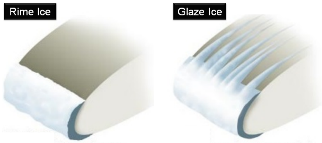
Fig. 3-4 Ice form at the leading edge of airfoil (left : rime ice, Right : glaze ice) [21]
