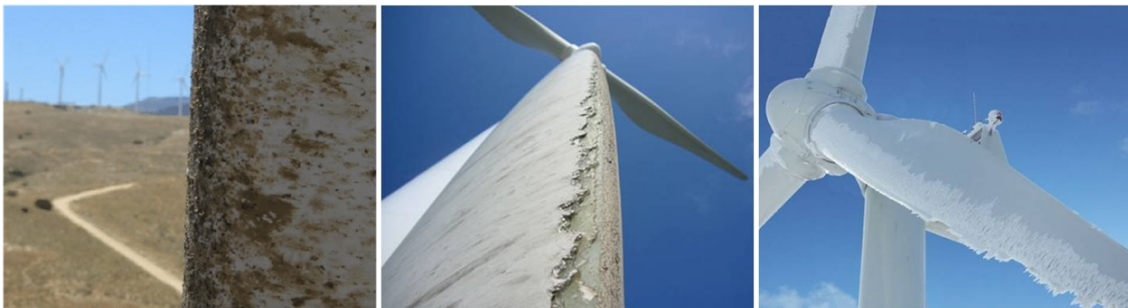
Fig. 1-1 Damages at the leading edge of wind turbine blades
