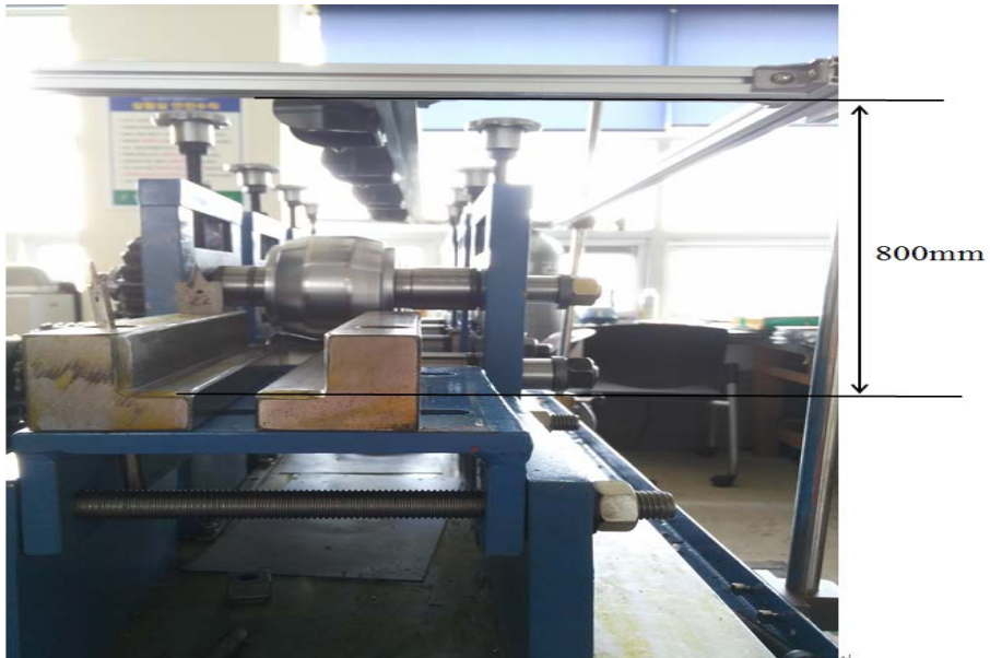
Fig. 42 The pre-heating height of the butane torch
