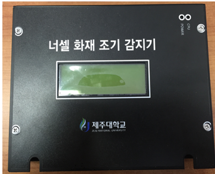
(a) Fire detection module
