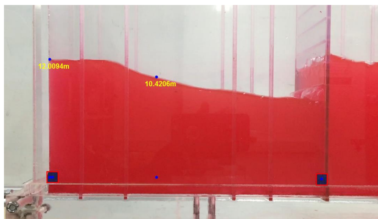
Fig. 3.7 Snapshot of the Image tracking for measuring water elevation and tank motion
