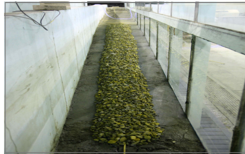
Fig 47. Rock berm model.
