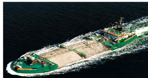
Fig 20. Side stone dumping. [14]
