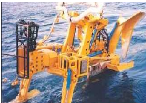
Fig 15. Burying (cable plough). [16]
