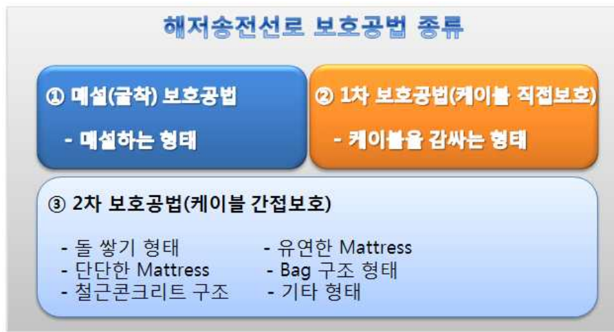
Fig 14. Undersea transmission line protection method type.
