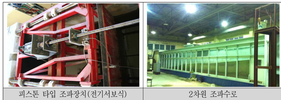
Fig 41. The facility of hydraulic model tests.
