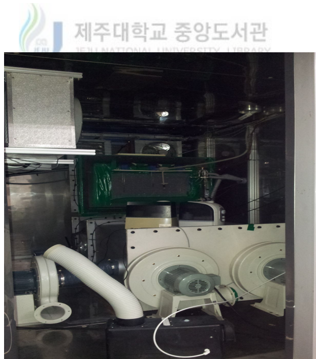
Fig. 5 Front view outdoor environmental chamber
