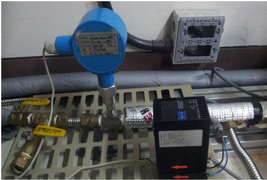
Fig. 16 Flowmeter and converter for flow measurement of stack simulator
