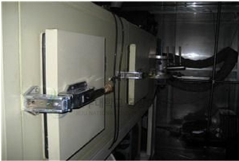
Fig. 4 Indoor environmental chamber and code tester
