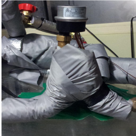
(a) 3RT EEV (Electronic expansion valve)
