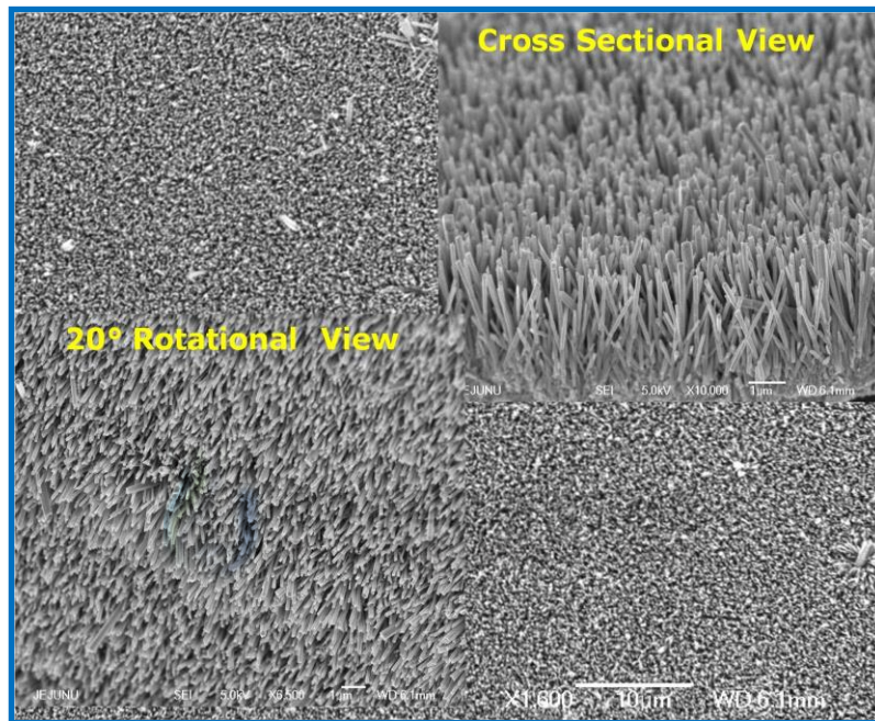
Fig.3.9. FE-SEM image of aligned nanowire array in-plane view. Insets cross sectional and 20^\circ tilted view.
