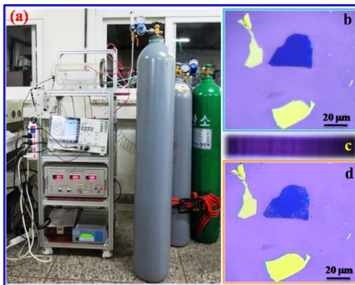
Fig.2.4. (a) Digital photograph of the DBD plasma reactor. (b and d) optical microscopic images of FLG graphene before and after plasma irradiation respectively. (c) Photograph of the generated argon plasma.
