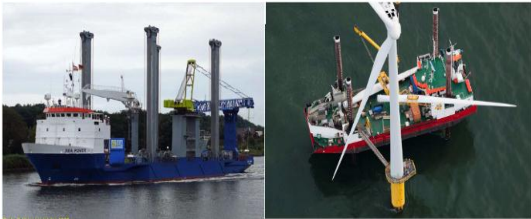
Figure 28 Jack-up vessel (Left: SEA POWER, Right: MV wind) [36].
