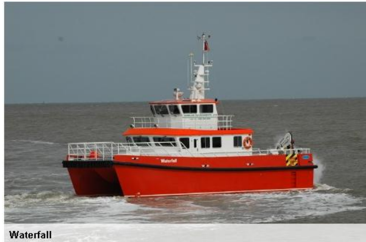
Figure 27 Example of a small access vessel (Waterfall) [36].
