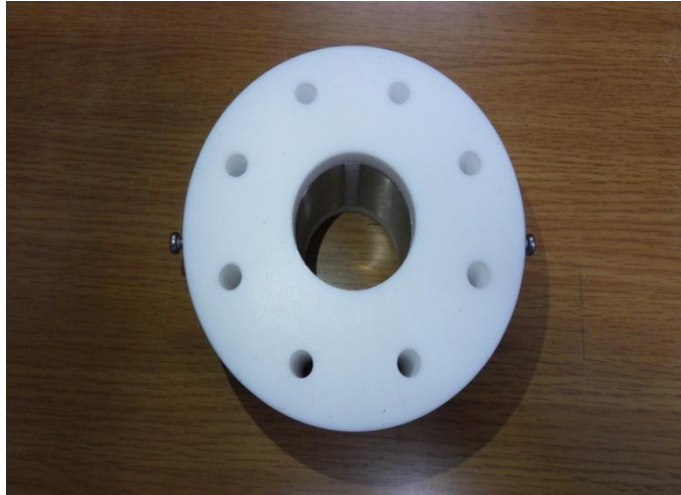
Figure 5.1. A conductance sensor for flow regime classification.
