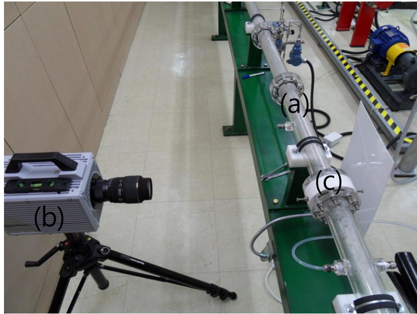
Figure 4.6. High-speed camera and impedance sensor installations. (a) horizontal pipe, (b) high-speed camera, (c) impedance sensor.
