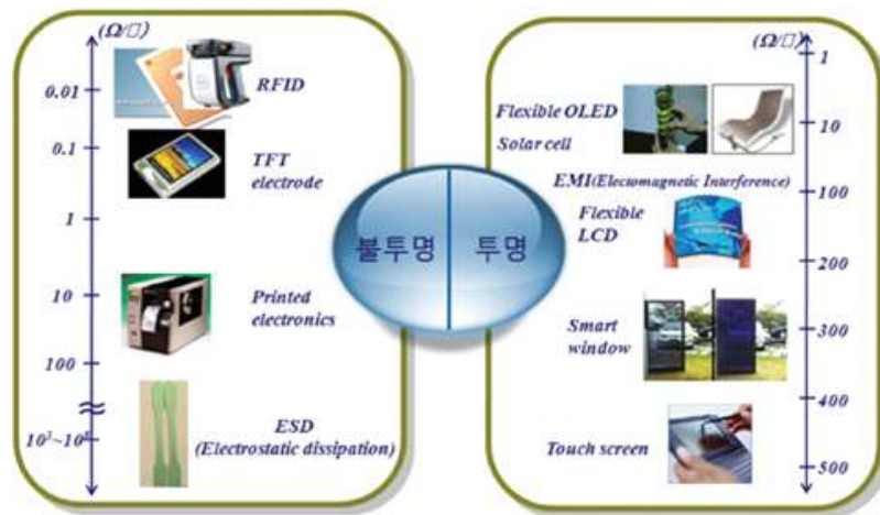
Fig. 6.1 Application of transparent conductive film
