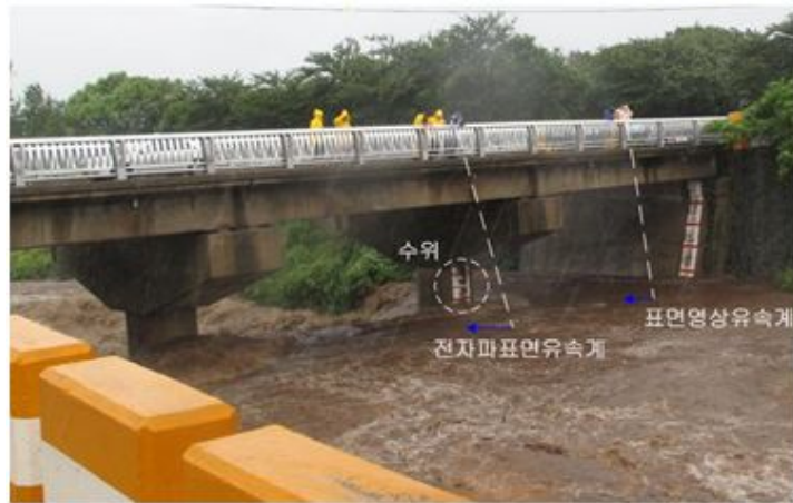
Fig. 3.5 Microwave water surface stream meter and LSPIV
