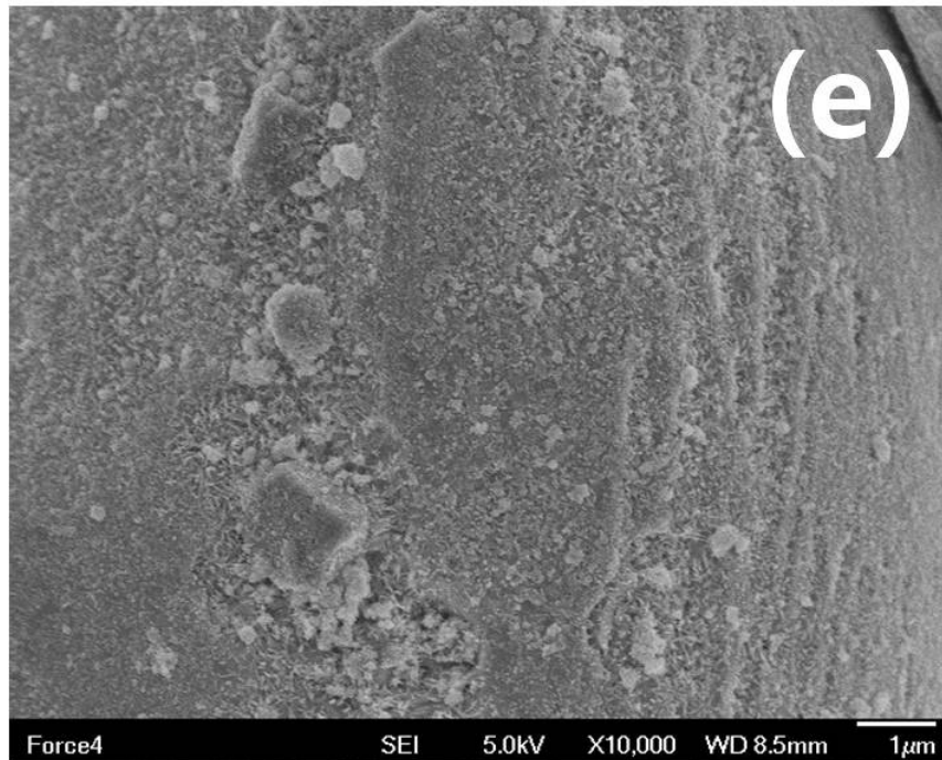
Figure 21. (e) HMDSO 1.65%; Toluene 1.09%; 20W.
