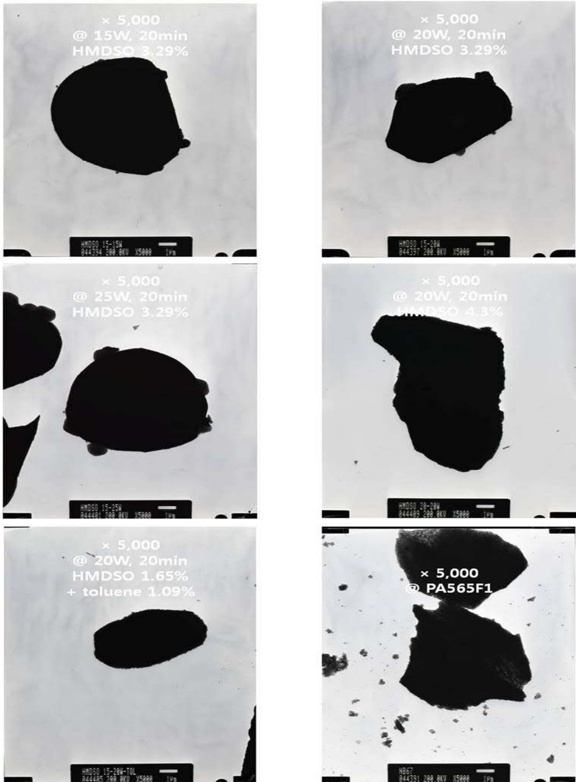
Figure 46. TEM images of the coating layers prepared under different conditions at the magnification of 5,000. (coating time: 20min; precursor: HMDSO and toluene)
