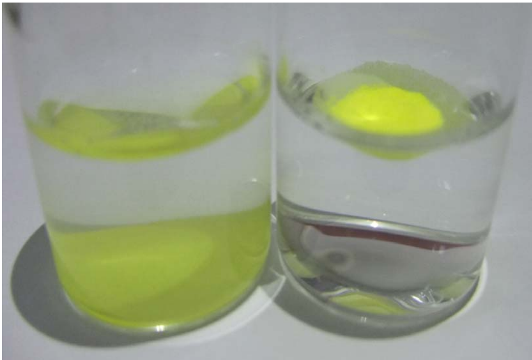
Figure 31. Comparison of the wettability for un-coated (left) and HMDSO-coated phosphor powder (right). (HMDSO content: 4.3%; coating time: 20 min; input power: 20 W)
