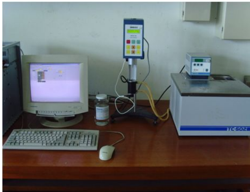
Figure. 14. The measurement experimental apparatus of viscosity.
