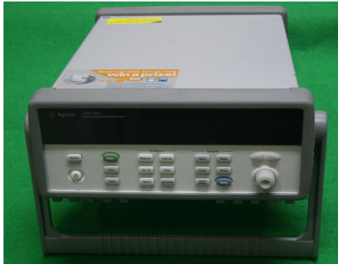
Figure 26. Photograph of data logger(34970A)
