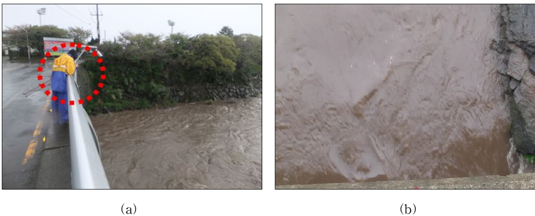
Fig. III-7. The shooting location for the analysis of the "STIV"(a) and the acquired images(b).
