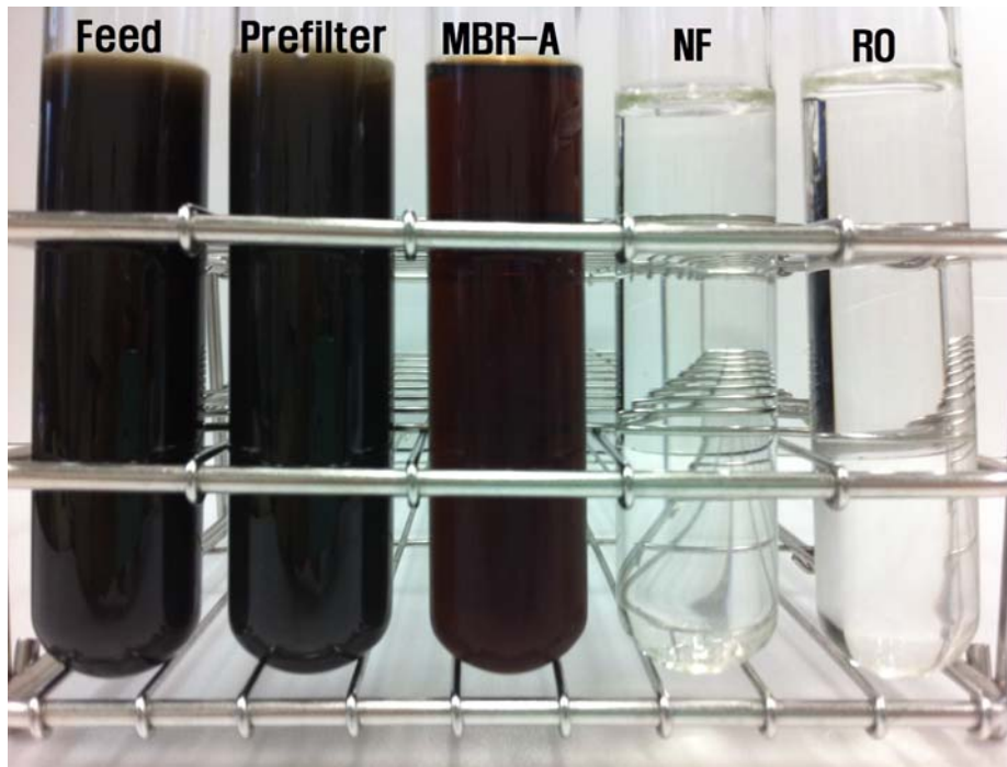
Fig. 33. Photograph of filtrate and permeate by 1\mu\text{m} cartridge filter, MBR-A, NF, and RO process.
