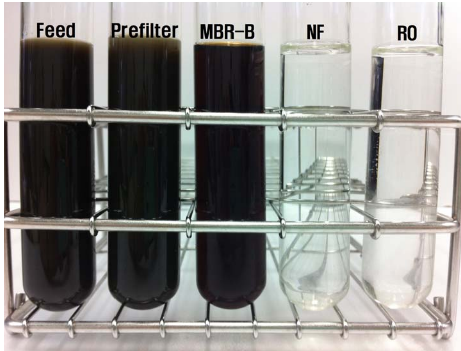
Fig. 34. Photograph of filtrate and permeate by 1\mu\text{m} cartridge filter, MBR-B, NF, and RO process.
