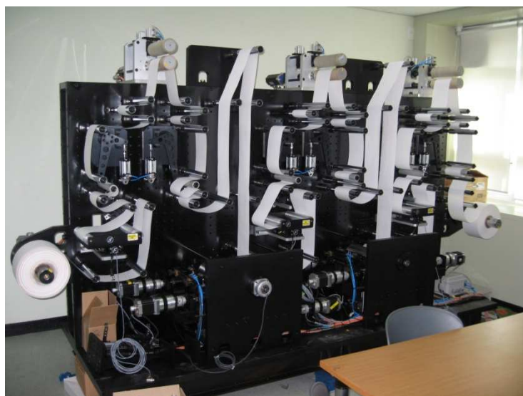
Figure 1.3: Offset-gravure R2R printing technology
