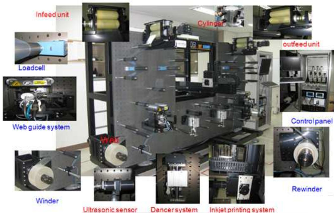
Figure 4.1: R2R web system based inkjet printing system at AMM Lab
